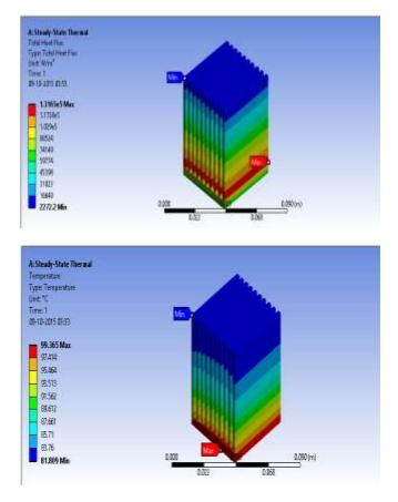
From the above plot it is observed that maximum and minimum temperatures on the heat sink. Max temperature=99.3650C
